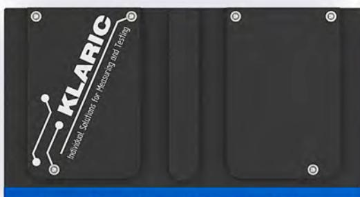
ETHERNET measuring module for measuring quiescent, operating and peak currents as well as voltage and temperature with KLARI-PROBES
